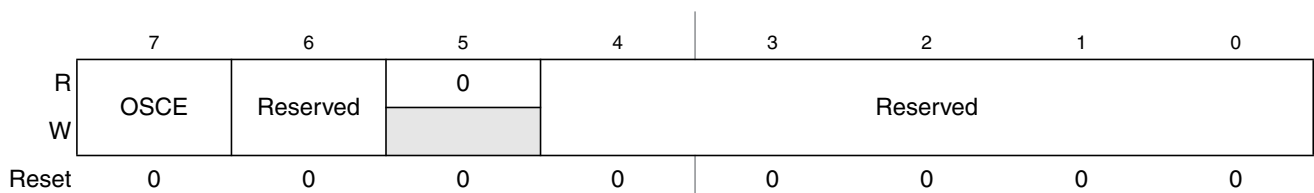
Figure 4-30. S12CPMU_UHV Oscillator Register (CPMUOSC)
