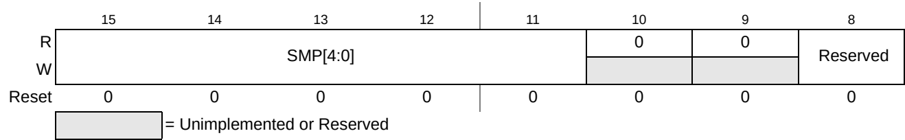
Figure 10-20. ADC Command Register 2 (ADCCMD_2)
