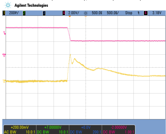
Figure 18 - Load transient V1, 244 to 122 A (500 µs/div) CH1: V1 (200 mV/div); CH4: I1 (100 A/div)
