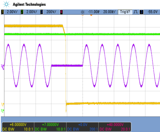
Figure 13 - AC drop out 40 ms, full load (20 ms/div) CH1: V1 (2 V/div); CH2: VSB (2 V/div); CH3: Vin (200 V/div)
