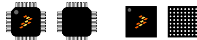
64-pin LQFP (LH) 10 x 10 x 1.4 Pitch 0.5 mm 64-pin MAPBGA (MP) 5 x 5 x 1.23 Pitch 0.5 mm
