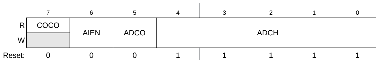
Figure 10-3. Status and Control Register (ADCSC1)
