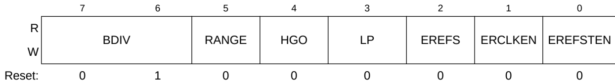
Figure 8-4. MCG Control Register 2 (MCGC2)
