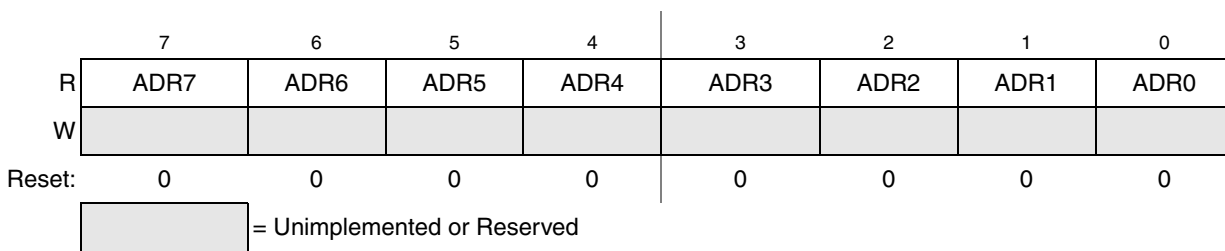
Figure 9-7. Data Result Low Register (ADCRL)
