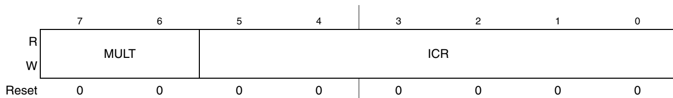
Figure 11-4. IIC Frequency Divider Register (IICF)
