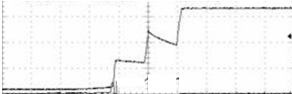
Figure 23. Supply Voltage Drop
