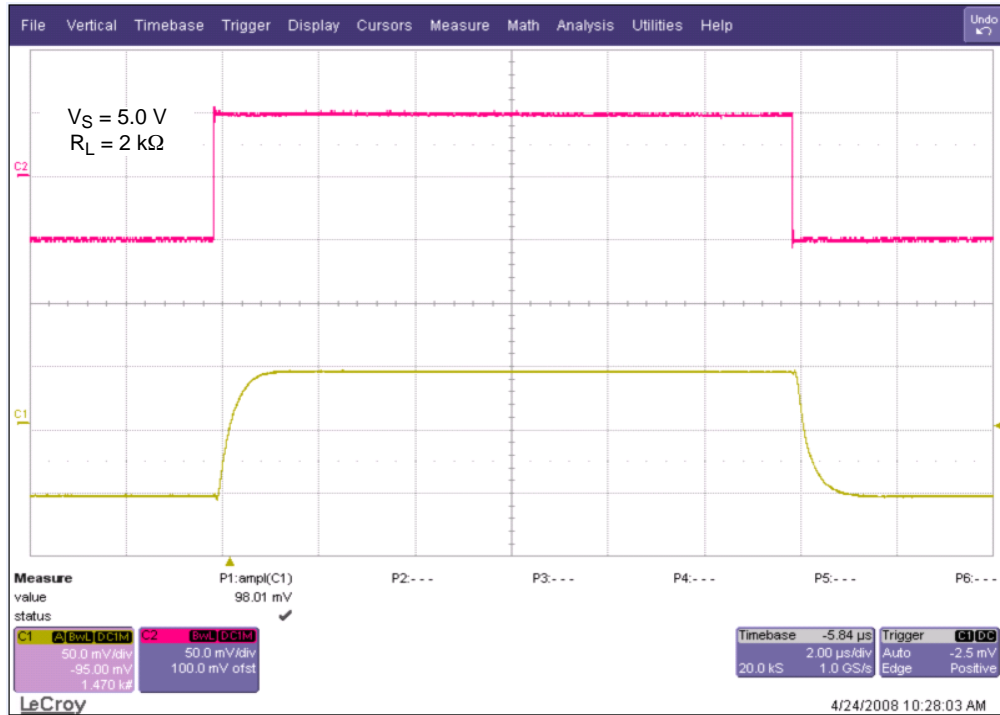
Figure 18. Small Signal Noninverting Response
