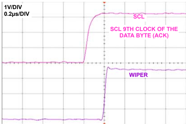
FIGURE 21. WIPER LARGE SIGNAL SETTLING TIME
