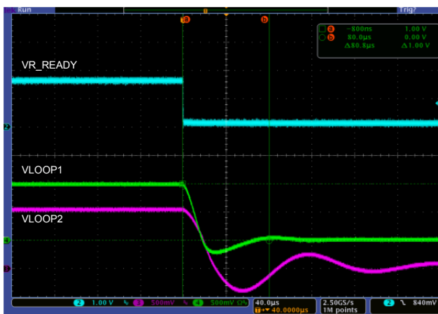
Figure 42: OVP - MOSFET latched on
