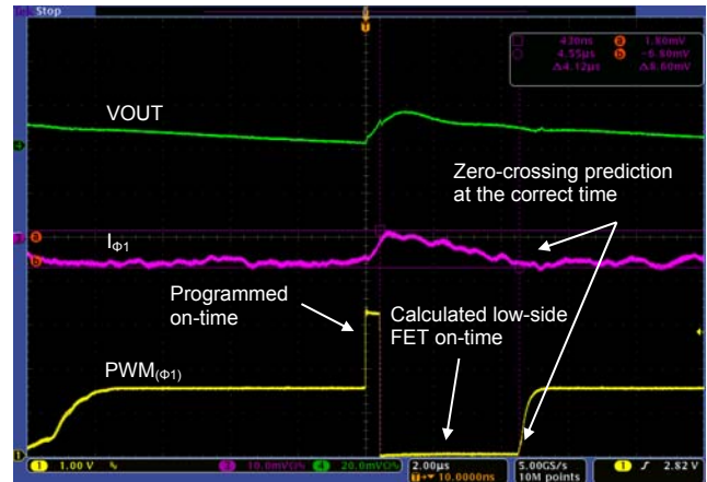
Figure 41: PS2 Active Diode Emulation Mode
