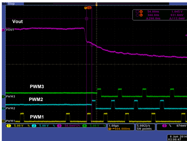
Figure 39: Phase Add 1\Phi \rightarrow 3\Phi
