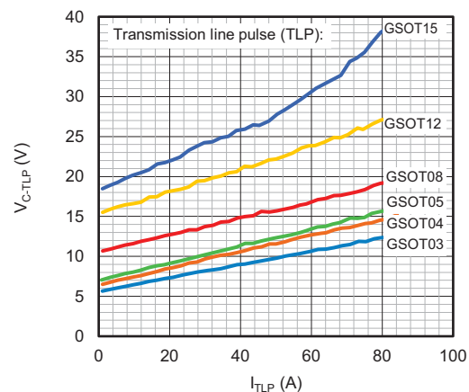
Fig. 6 - Typical Clamping Voltage vs. Peak Pulse Current
