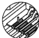
Uplift of the conductor
