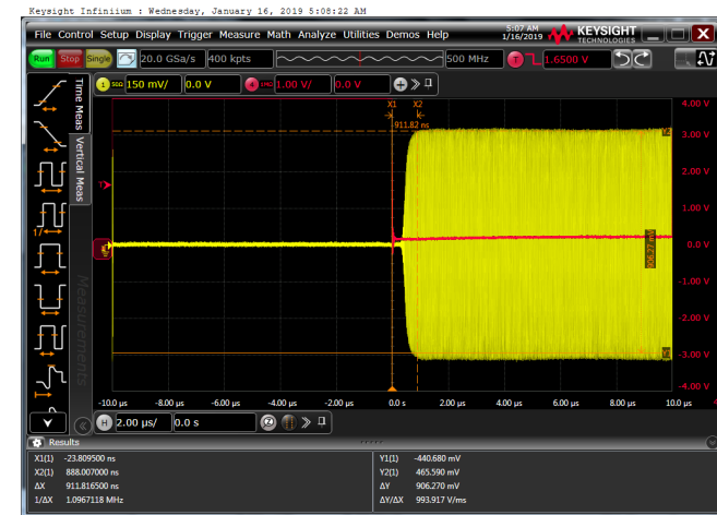
Figure 25. 6dB Gain Reduction Transient Time
