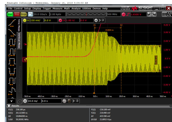
Figure 25. 6dB Gain Reduction Transient Time
