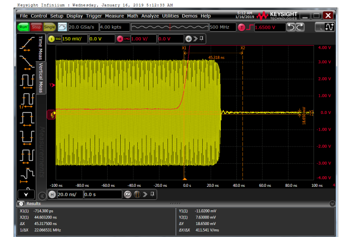
Figure 26. 6dB Gain Increase Transient Time
