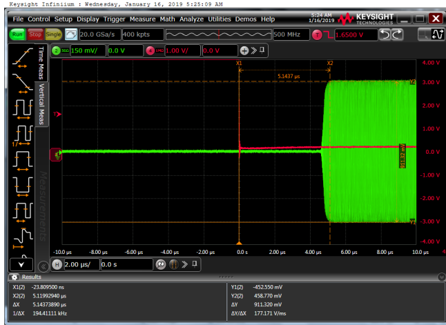
Figure 23. Standby to RX Mode Transient Time
