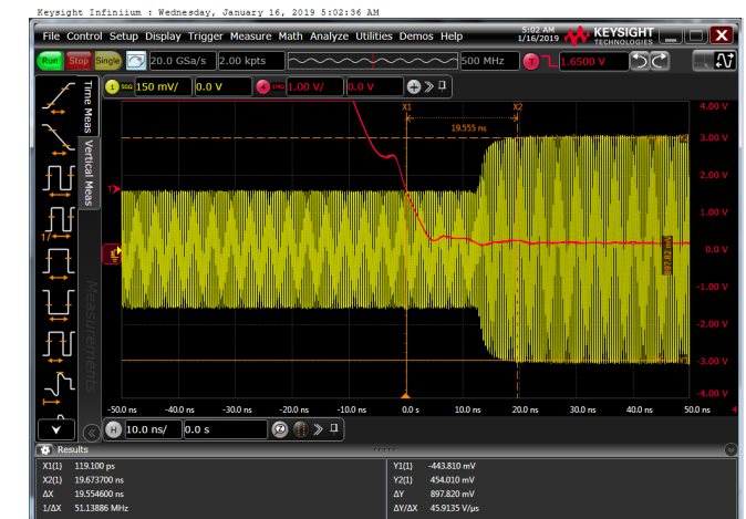
Figure 26. 6dB Gain Increase Transient Time
