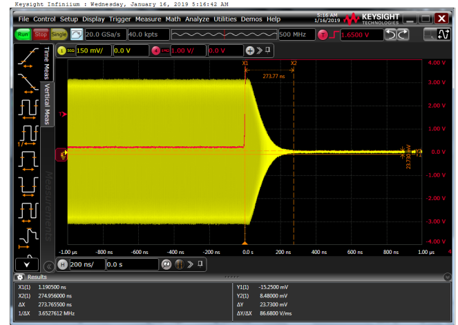
Figure 24. RX Mode to Standby Transient Time
