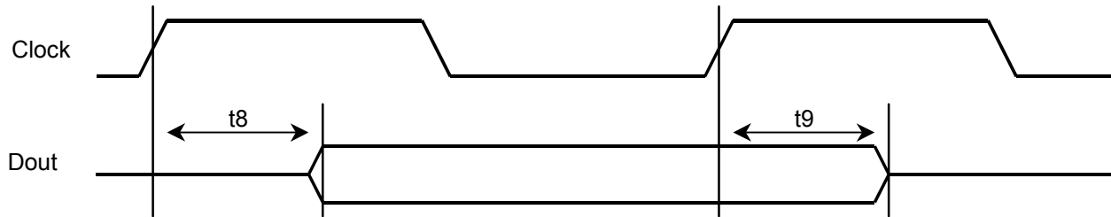
Figure 18-5. To/From High-Z Delay Definitions (Rising Clock Edge)
