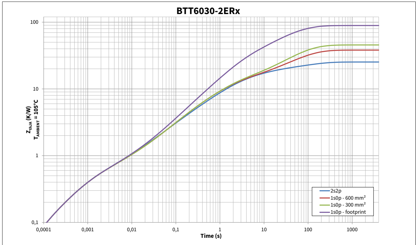
Figure 6 Typical Thermal Impedance. 2s2p set-up according Figure 4
