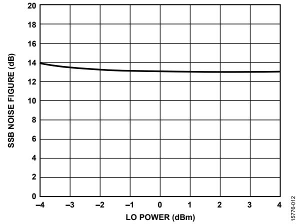
Figure 12. SSB Noise Figure vs. LO Power, RF Frequency = 18 GHz
