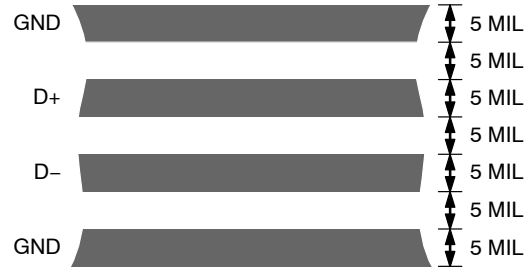
Figure 28. Arrangement of Signal Tracks
