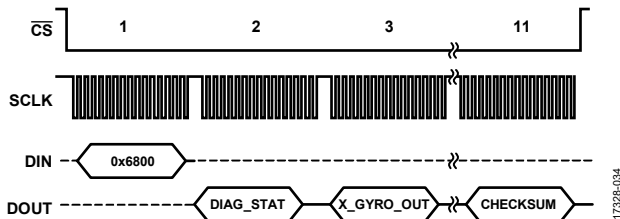
Figure 42. Burst Read Sequence with BURST_SEL = 0
