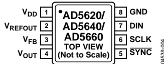
Figure 4. MSOP Pin Configuration
