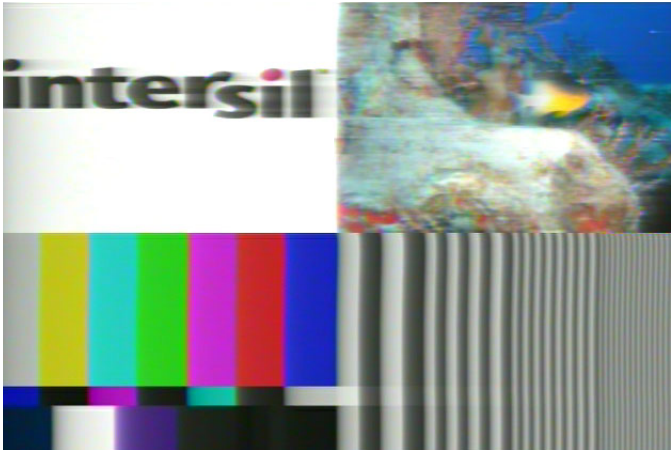
FIGURE 41. TEST PATTERN IMAGE AFTER 6000 FEET OF UNCOMPENSATED RG-59 COAX
