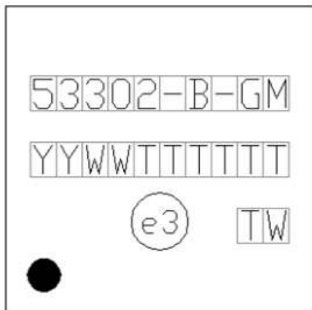
Figure 8.4. Si53302 Top Marking
