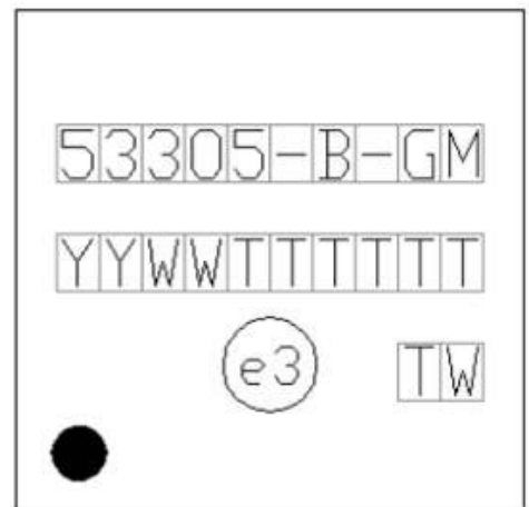
Figure 8.6. Si53305 Top Marking
