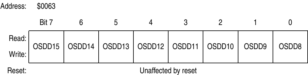
Figure 18-7. OSD Data Register High (OSDDRH)
