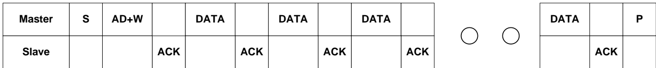
Figure 1-16: I 2 C write cycle
