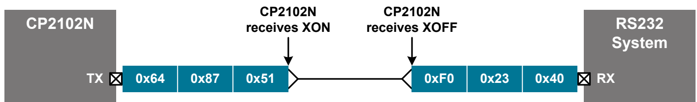
Figure 4.2. Software Flow Control Timing Diagram
