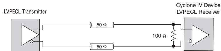
Figure 6-19. LVPECL DC-Coupled Termination (1)
