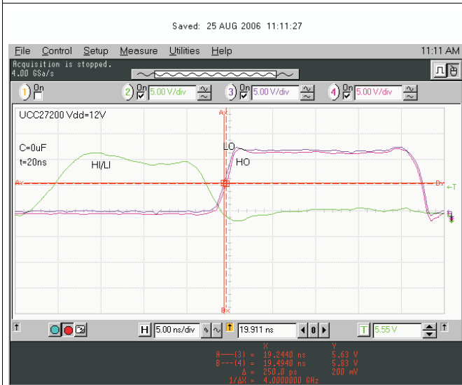
Figure 32. 20-ns Input Pulse Delay Matching
