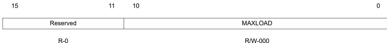
Figure 17-33. USB Maximum Transmit Data Endpoint n Registers (USBTXMAXP[ n ])
