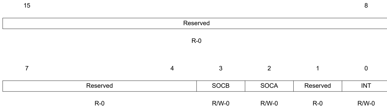
Figure 3-104. Event-Trigger Clear Register (ETCLR)
