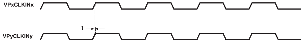
Figure 6-31. Video Port Dual-Display Sync Timing
