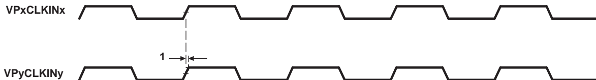
Figure 5-61. Video Port Dual-Display Sync Timing
