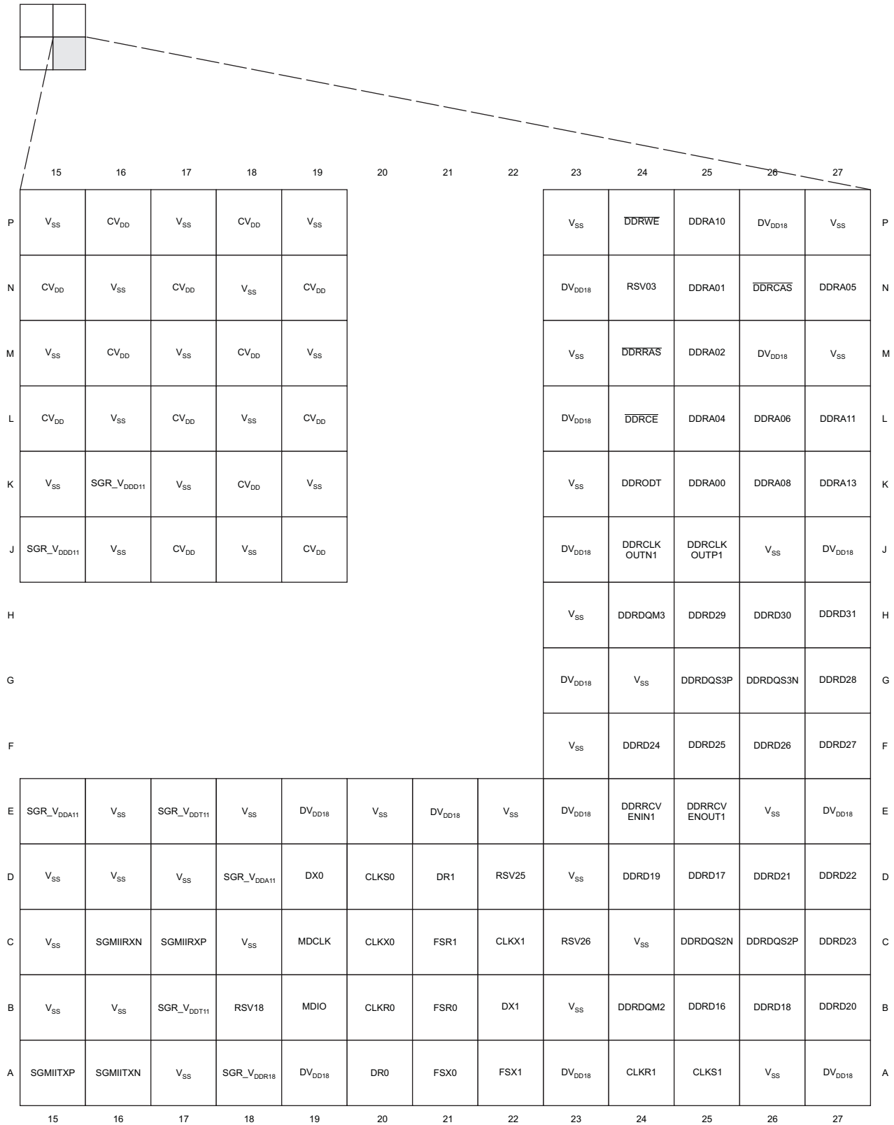
Figure 2-4. C6474 Pin Map (Bottom View) [Quadrant C]
