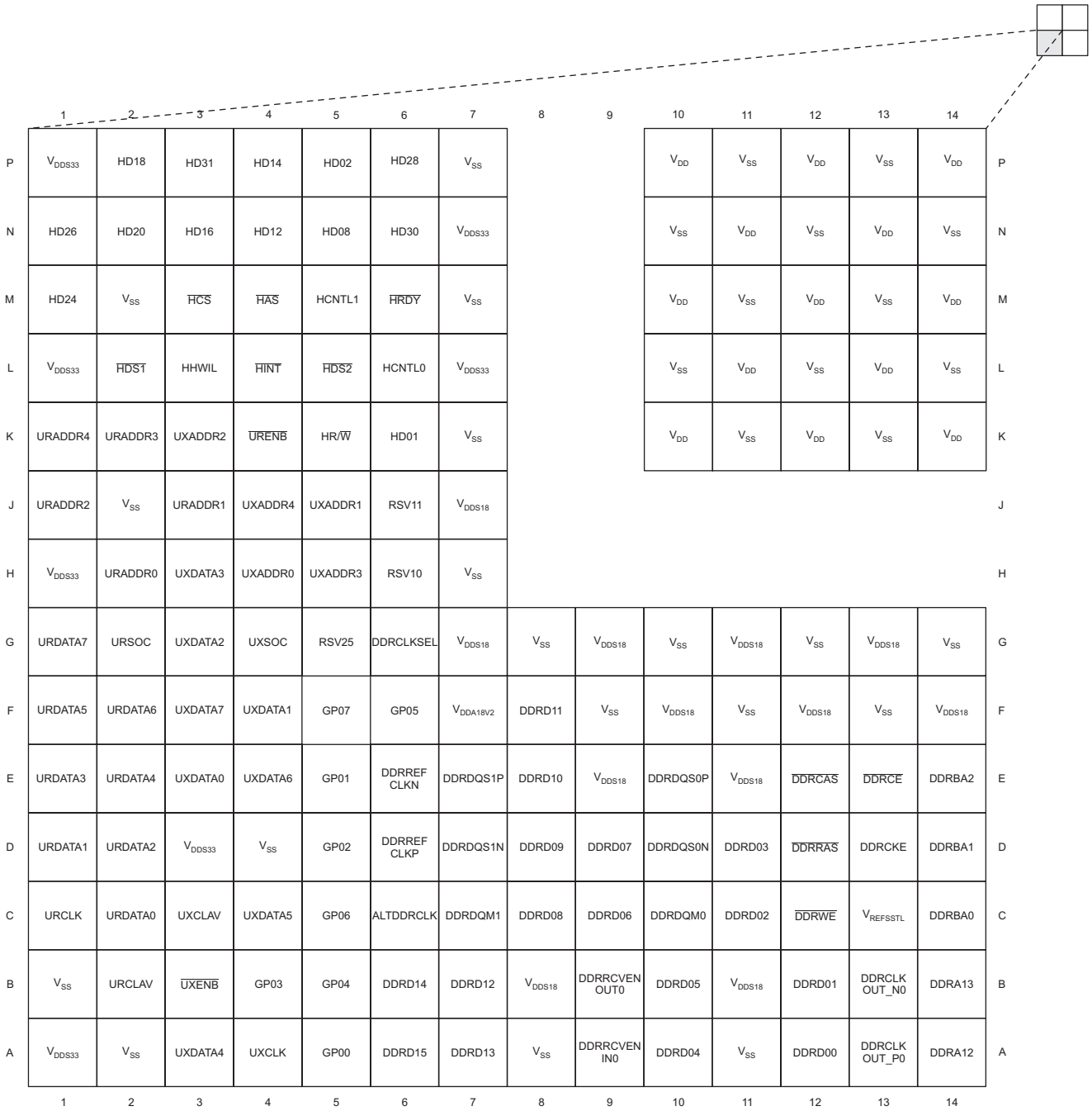
Figure 2-5 TMS320C6457 Pin Map (Bottom View) [Quadrant D]
