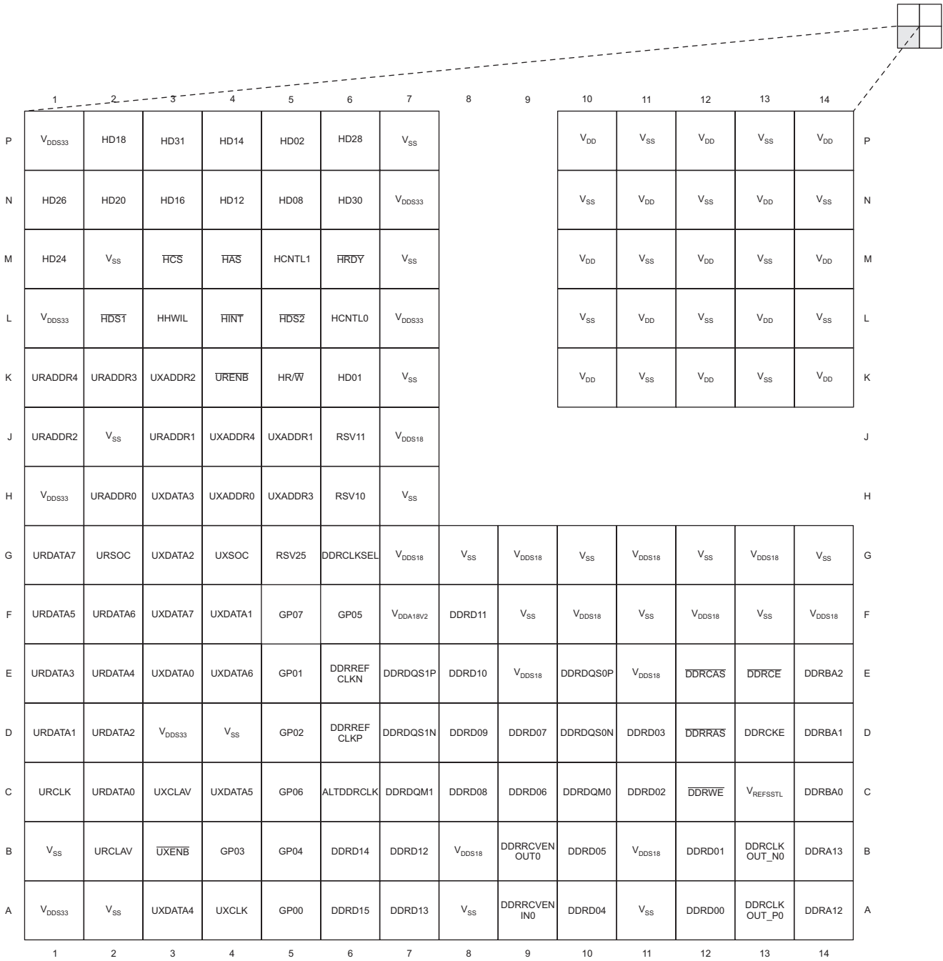
Figure 2-5 TMS320C6457 Pin Map (Bottom View) [Quadrant D]
