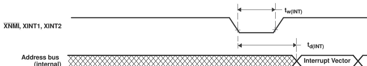
Figure 7-15. External Interrupt Timing
