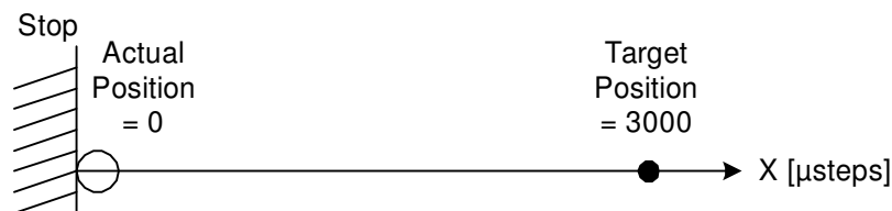
Figure 23: Positioning Example: Situation after reference search
