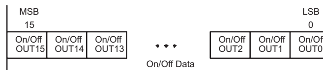
Figure 8. On/Off Data Format
