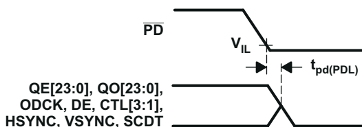
Figure 8-7. Delay From \overline{PD} Low to Hi-Z Outputs
