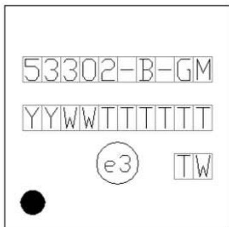
Figure 8.4. Si53302 Top Marking
