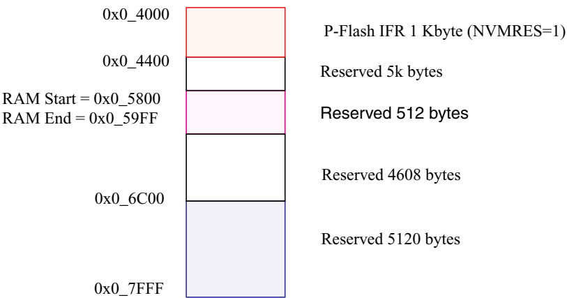
Figure 24-3. Memory Controller Resource Memory Map (NVMRES=1)
