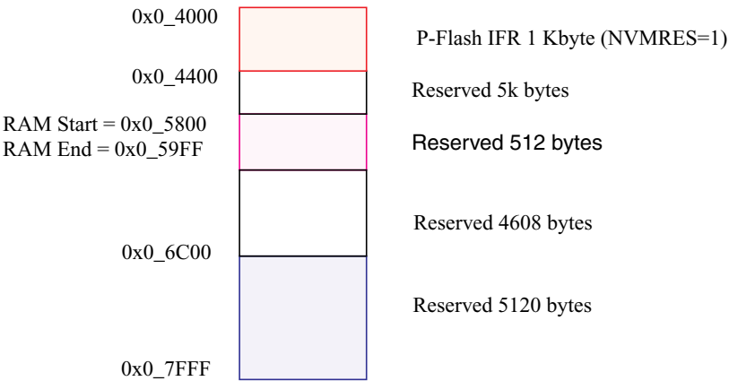
Figure 29-3. Memory Controller Resource Memory Map (NVMRES=1)
