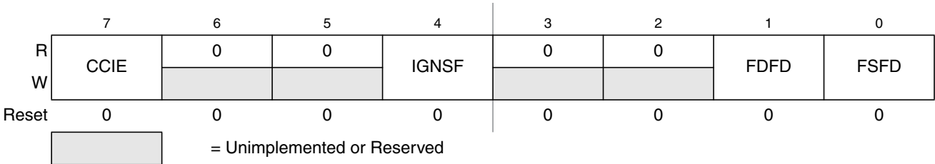
Figure 26-9. Flash Configuration Register (FCNFG)
