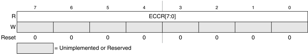
Figure 25-21. Flash ECC Error Results Low Register (FECCRLO)
