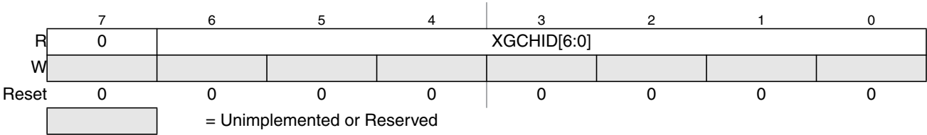
Figure 10-4. XGATE Channel ID Register (XGCHID)
