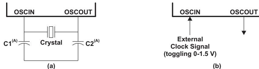
Figure 5-5. Recommended Crystal/Clock Connection
