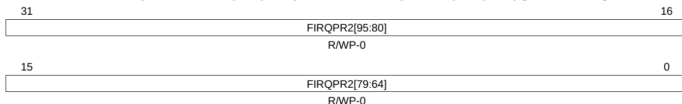
Figure 15-19. FIQ/IRQ Program Control Register 2 (FIRQPR2) [offset = 18h]
