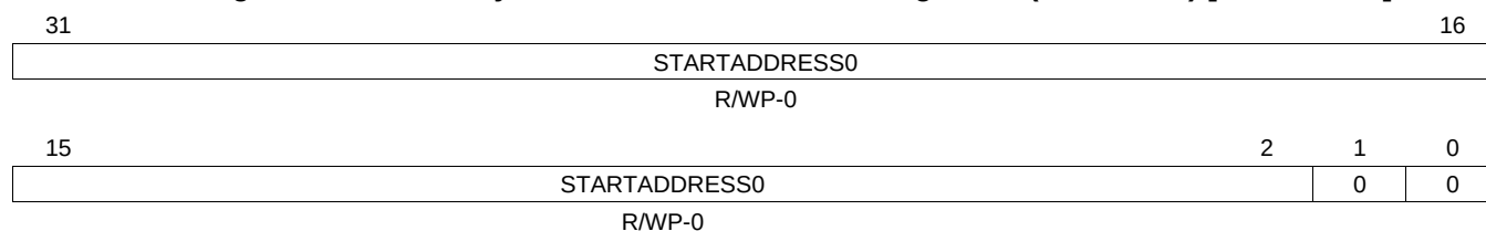
Figure 21-40. Memory Protection Start Address Register 0 (HTU MP0S) [offset = 74h]
