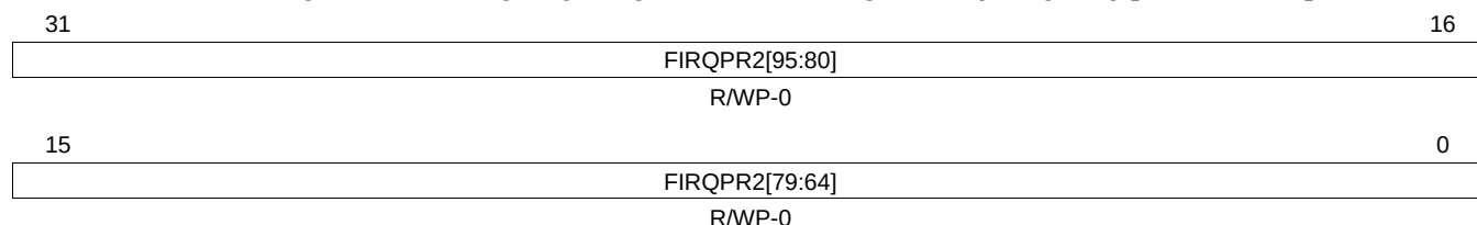
Figure 15-19. FIQ/IRQ Program Control Register 2 (FIRQPR2) [offset = 18h]
