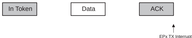
Figure 29-51. Non-Isochronous, Non-Control OUT Transaction Phases and Interrupts
