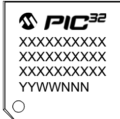
64-Lead QFN (9x9x0.9 mm)
