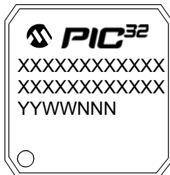
100-Lead TQFP (12x12x1 mm)
