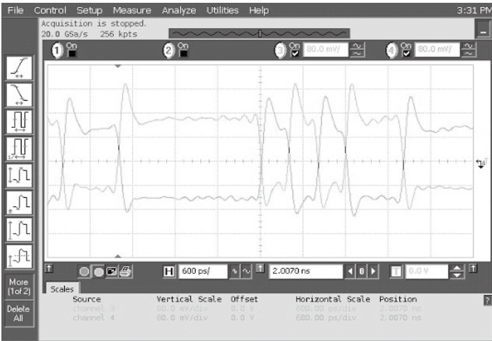
Data Waveforms, 3.0Gbps (left) & 6.0Gbps (right)
