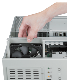
Easy-to-maintain cooling fan
