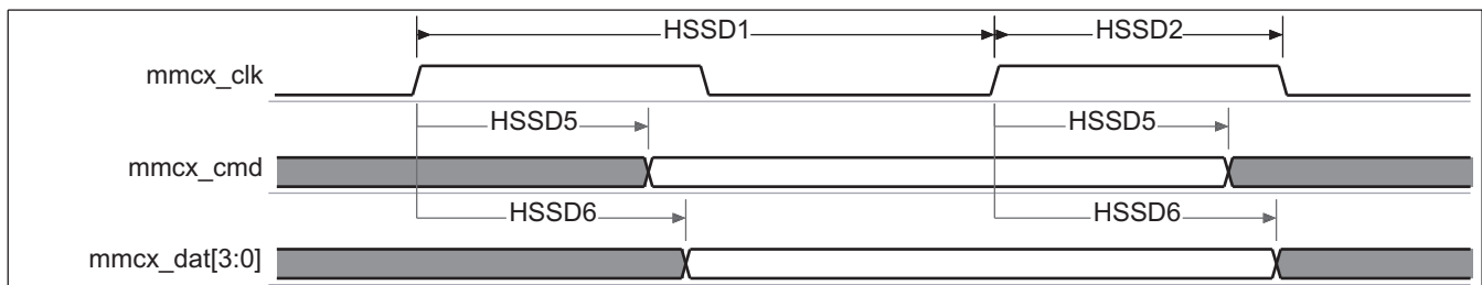
Figure 6-65. MMC/SD/SDIO – High-Speed SD Mode – Data/Command Receive
