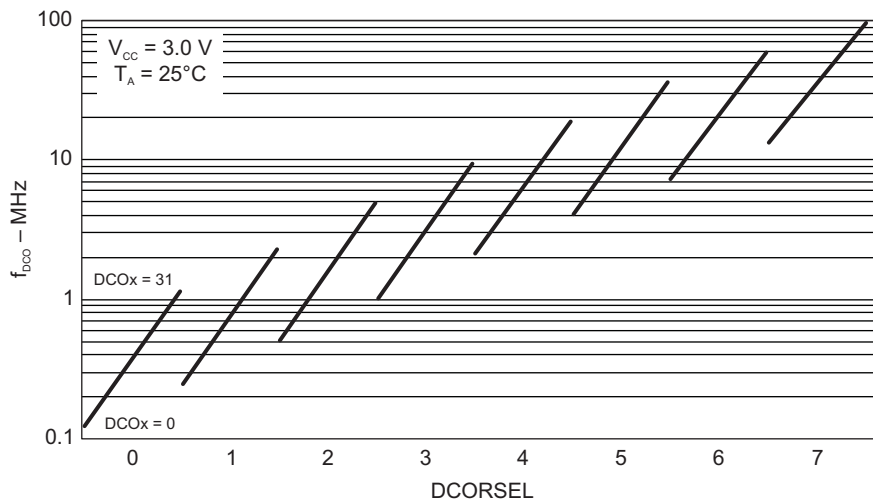
Figure 5-10. Typical DCO Frequency
